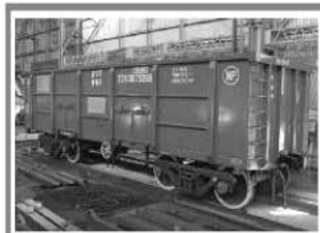
Stainless Steel Railway Wagon Manufactured at Howrah Work Shops
